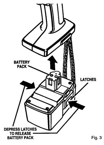
Make sure the latches on each side of your battery pack snap in place and battery pack is secured in drill before beginning operation.
